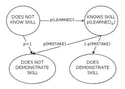
Figure 4: The Bayesian network skill assessment algorithm; an assessment of each skill is determined by an independent network in the form above. The upper nodes are internal states of the algorithm and the lower nodes correspond to the robot's observations of the user. For details see Section 4.2.
